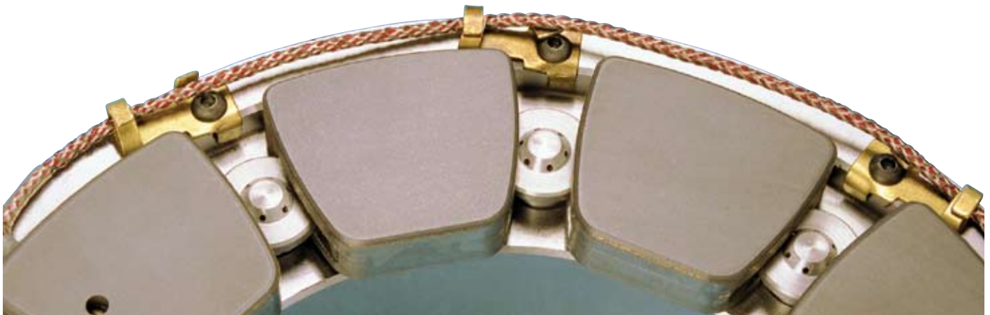
Polymer-lined pads are available for non-equalized and equalized tilt-pad thrust bearings as well as tilt-pad journal bearings. Designs can include either flooded or 'Directed Lubrication' configurations with provisions for RTD's or thermocouples for temperature measurement. The photo above shows a 215 mm (8.5 inches) thrust bearing with 'Directed Lubrication' and temperature sensors to resist heat soak in a high-speed gas turbine.
