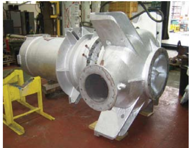
"Wet wound" heater lift pumps used in large power stations are being upgraded with solid polymer thrust bearings to replace ferrobestos materials. (Photo courtesy of Weir Engineering Services Ltd.)
