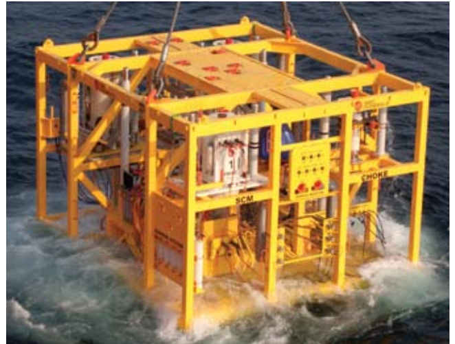
A subsea module containing two water-injection pumps with polymer thrust and journal tilt-pad bearings. (Photo courtesy of Framo Engineering AS.)
