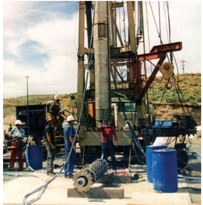
A 2,200 horsepower water-filled motor with a ceramic thrust bearing operating in a Nevada gold mine.
